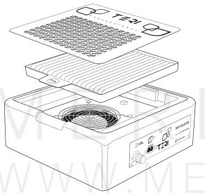
Warning! It is forbidden to switch on the dust collector without a filter! It is also forbidden to turn the filter over during operation! Turning the filter over may cause the malfunction of internal mechanisms, as well as blow the dust out of the filter spraying it around.
